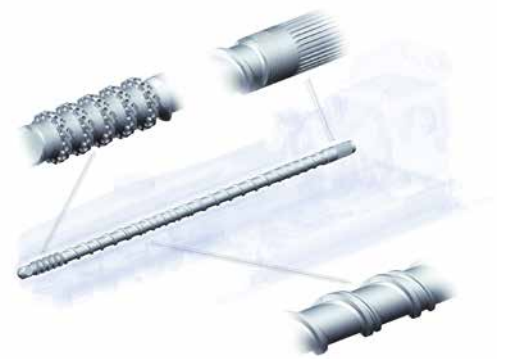
> Ideal proportions: Screw length to diameter ratio (L/D) = factor 30.
