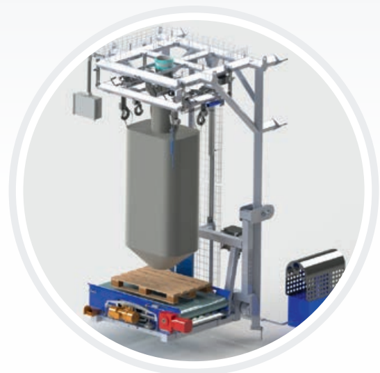
› BigBag filling station
